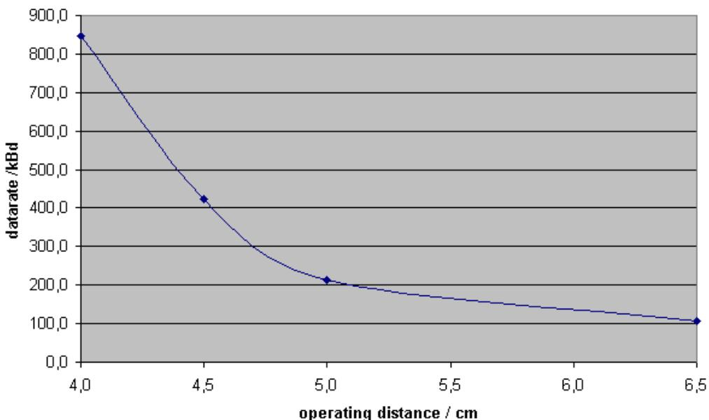
**Fig 4. Operating distance versus bit rates (example)**
