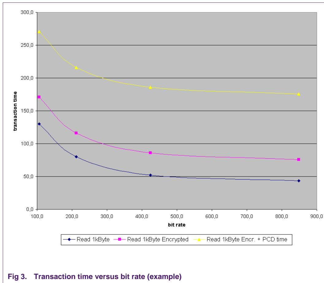
**Fig 3. Transaction time versus bit rate (example)**
