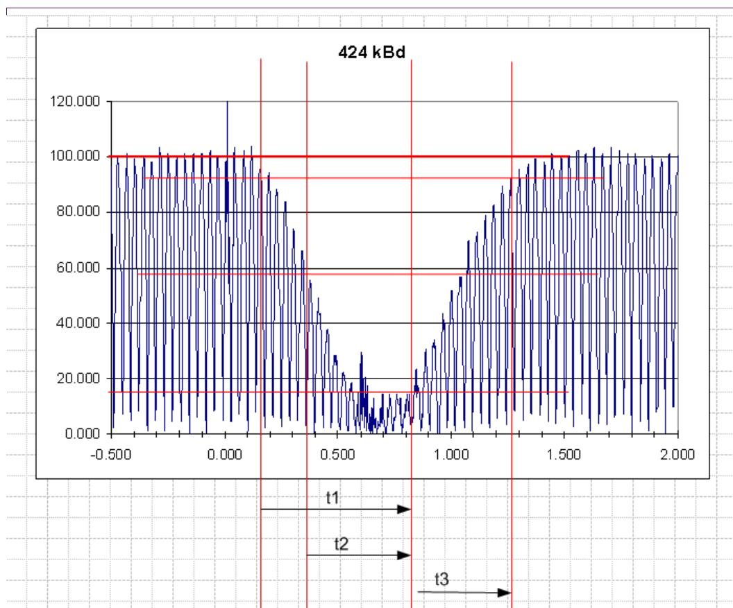
Fig 2. Typical pulse shape example for 424 kbit/s
